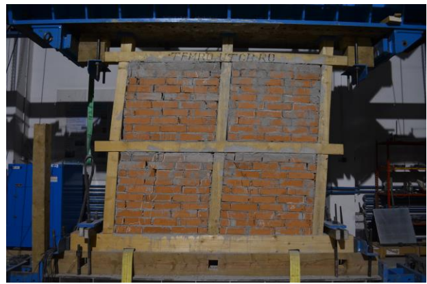
Figure 10: Specimen's last cycle at 6 % drift
