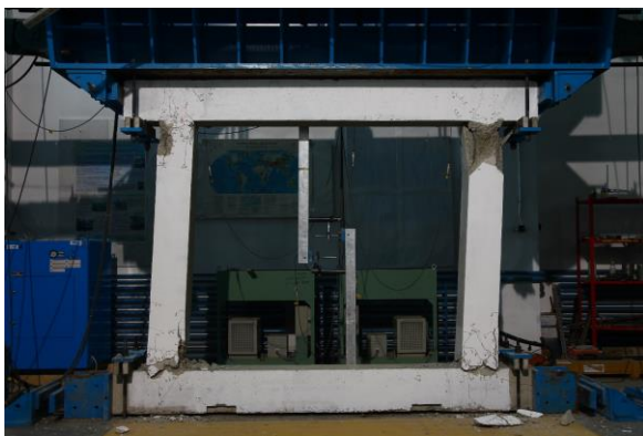
Figure 11. Frame's (S1-F) failure at 2 % drift (left) and hysteric curve
