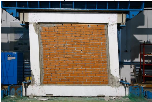
Figure 12. Frame's (S2-FTCM) failure at 4% drift (positive cycle) (left) and hysteric curve (right)
