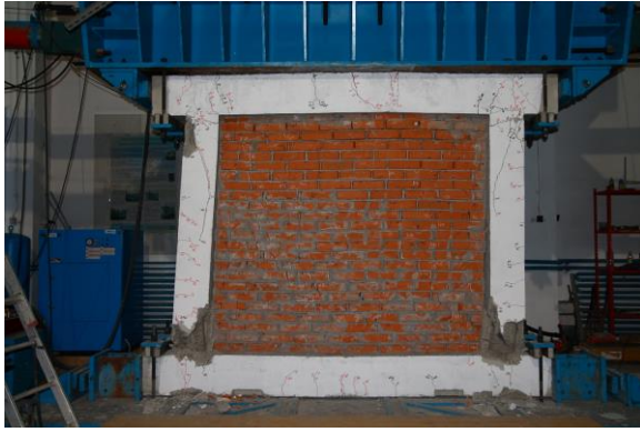
Figure 13. Frame's (S3-FM) failure at 3% drift (left) and hysteric curve (right)
