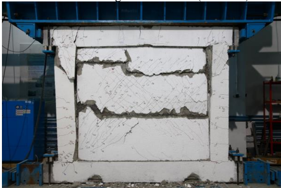
Figure 15. Frame's (S5-FMFC) failure at 1.5 % drift (left) and hysteric curve (right)
